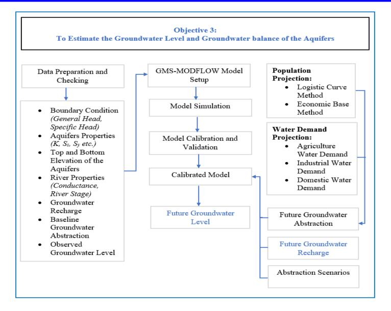
a. Groundwater(GW) Model to calculate GW Level and GW Balance
